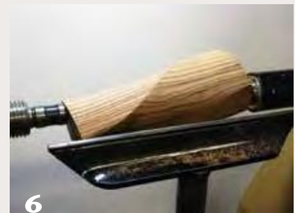
Mount and turn the spindle on three axes to produce a twist.
