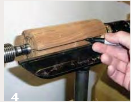
Extend the section lines down the cylinder to the opposite end, either freehand or with the aid of the toolrest. Locate and punch the three turning points at the opposite end, and label them as you did the first end.
