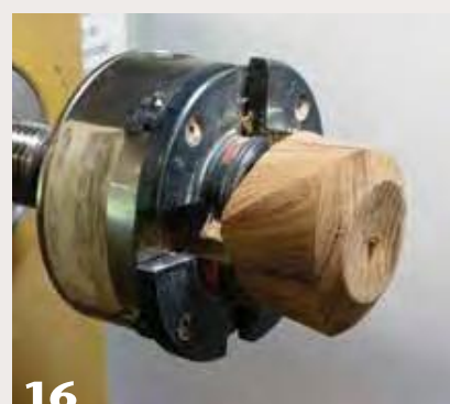
16 Reverse-mount the holder, using the chuck in expansion mode, to complete the bottom.
