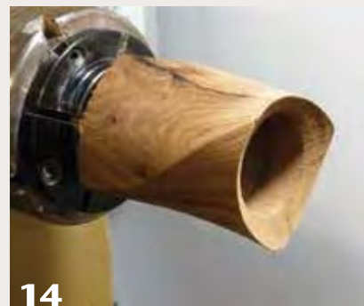
14 Use a Forstner bit to drill into the spindle deep enough to allow the tea light candle to sit all the way in and flush with the top.
