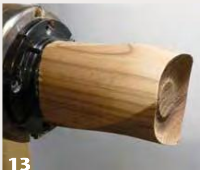
13 Begin a tea light holder by turning a concave shape at the end of the twisted spindle.
