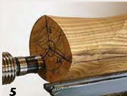
Mount and turn the spindle on three axes to produce a twist.
