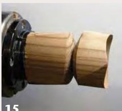
15 Part off the tea light holder by forming a concave area at the bottom.
