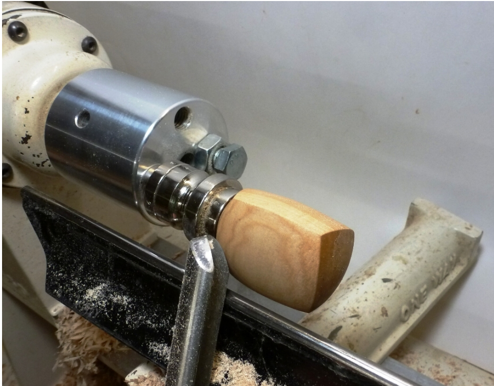
Three Sided Stopper, turned on the stopper mandrel with the Multi-port Holder
