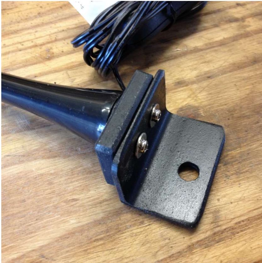
Photo 2 – Detail of Spacer and Angle Mount
